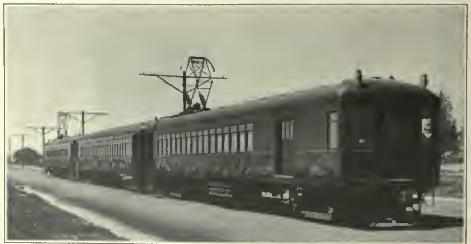
FIG. 537. MULTIPLE-UNIT TRAINS. Multiple-Unit Train for 1,200-Volt Direct Current Overhead Contact Operation, Southern Pacific Railroad.
